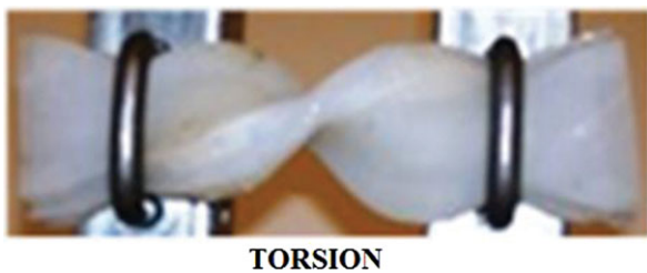
Fig. 2. Elastically deformed robot body.
