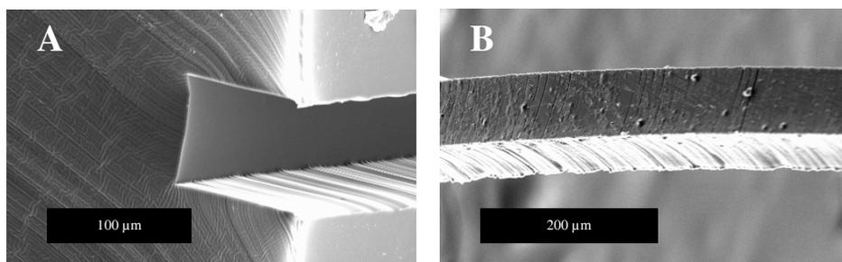
**Figure 4:** SEM image A on the left is showing a PDMS casting channel with width and height dimensions of approximately  $100 \mu\text{m} \times 100 \mu\text{m}$ . Image B on the right is showing a single casted silk fiber with the same dimensions.
