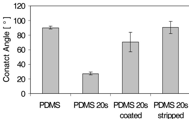
**Figure 2:** The bar graphs indicate contact angle measurements of silk solution droplets on treated and untreated PDMS surfaces (mean value  $n=3$ ). Black bars indicate standard deviation. *20s* refers to oxygen plasma treatment for duration of 20 seconds. *Coated* refers to a deposited a thin silicone grease film on the surface. *Stripped* refers to removal of the top most layer of PDMS surface with a razor blade.
