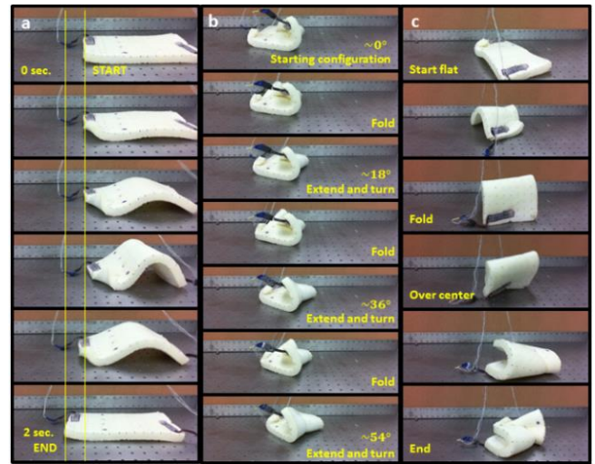
Figure 1: The motors were actuated with game controller inputs to an Arduino-controlled array of motor drivers. a) The robot demonstrating an inching gait. Forward speed is approximately 13 mm per second. b) The robot demonstrating a turning gait. Each motion of this configuration produces about 18 degrees of rotation. c) The robot folding and flipping end-over-end.
